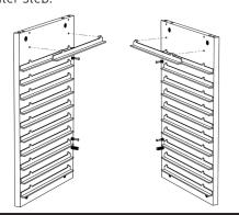
5.) Lay the back panel on the floor with the Cam Locks facing up. Attach both side panels to the back panel by sliding the Quick-Fit Dowel into the pre-drilled holes on the edge of the back panel. Tighten the Cam Locks by turning clockwise. Complete this step twice to prepare two identical assemblies.
