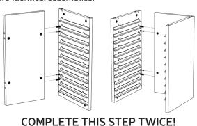
**6.)** Flip over one of the assemblies from step 5 and attach the bottom panel, tightening the Cam Locks in the same manner. Ensure that Rails match the orientation shown below.
