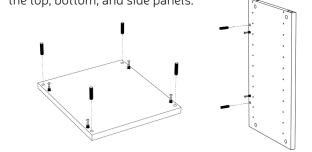
Insert the Cam Locks into the larger holes on the back and side panels. Make sure the arrow on the Cam Lock is pointing towards pre-drilled hole in edge of panel.
