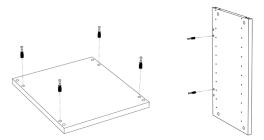
2.) Insert the Wood Dowels into the <u>outside</u> holes shown on the top, bottom, and side panels.
