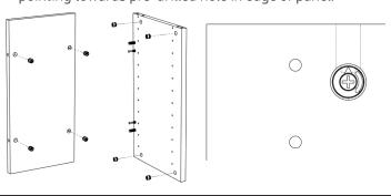
Attach Rails to left and right side panels, saving the top Rail for a later step.
