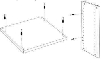
2.) Insert the Wood Dowels into the <u>outside</u> holes shown on the top, bottom, and side panels.
