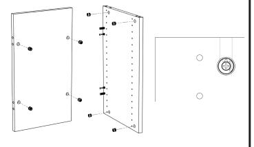
**4.)** Lay the back panel on the floor with the cam locks facing up. Attach both side panels to the back panel by sliding the cam lock bolts into the pre-drilled holes on the edge of the back panel. Tighten the cam locks by turning clockwise. Complete this step twice to prepare two identical assemblies.
