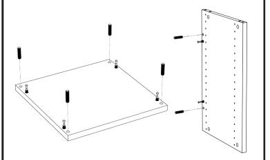
**3.)** Insert the cam locks into the larger holes on the back and side panels. Make sure the arrow on the cam lock is pointing towards pre-drilled hole in side of panel.
