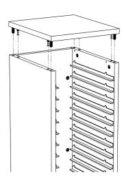
**7.)** Flip the cabinet over and attach the bottom panel.
