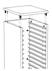
**8.)** Skip this step if you did not purchase Casters. Attach optional Casters using the pre-drilled holes. Be sure to lock Casters before flipping cabinet back over.
