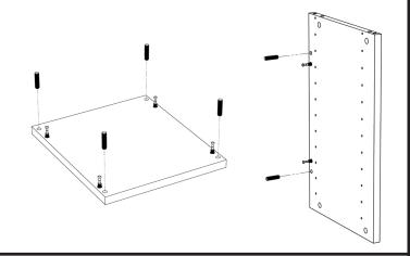
**3.)** Insert the Cam Locks into the larger holes on the back and side panels. Make sure the arrow on the Cam Lock is pointing towards pre-drilled hole in edge of panel.
