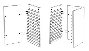
**6.)** Attach the top panel, tightening the Cam Locks in the same manner. Ensure that Rails match the orientation shown below.
