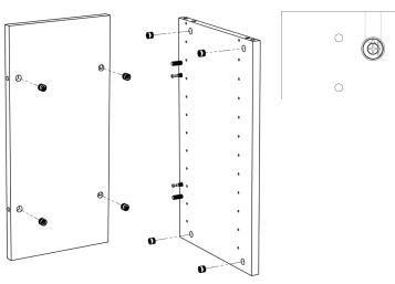
**4.)** Attach Rails to left and right side panels, saving the top Rail for a later step.
